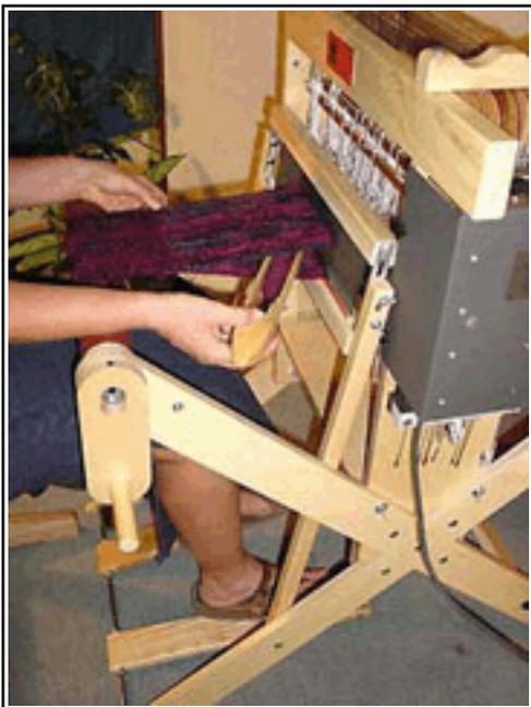
*Inserting the Shuttle*
